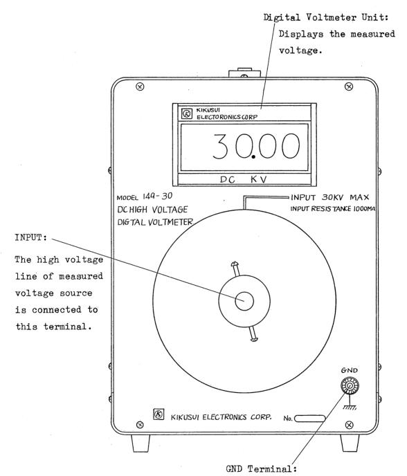
Connected to the low voltage line of measured voltage source and to the earth ground.
